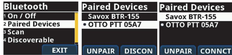
To scan for available Bluetooth devices, select the Scan menu option (Figure 4.9). Select a device name and press the Pair soft button to pair the device with the radio.
