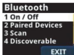
A list of paired devices can be viewed by accessing the Paired Devices menu option (Figure 4.8). Paired devices can be unpaired and connected or disconnected, depending on current connection status.
