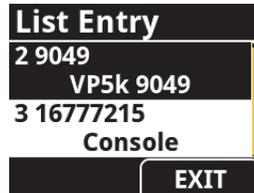
The radio user can enter Unit IDs manually on the **Direct Entry** menu (Figure 4.25). To enter **Direct Entry**, the **Recipient Usage** must be set to **Unlimited**.
