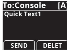
Pressing the **SEND** soft button sends the quick text immediately and takes you back to normal operation. Pressing the **Select/Enter** button takes you to the **Compose** menu with the quick text already entered.
