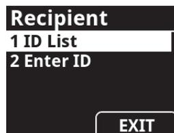
Radios listed in the system's Call List can be chosen on the **List Entry** menu (Figure 4.24). To enter **List Entry**, the **Recipient Usage** must be set to **List Only** or **Unlimited**.
